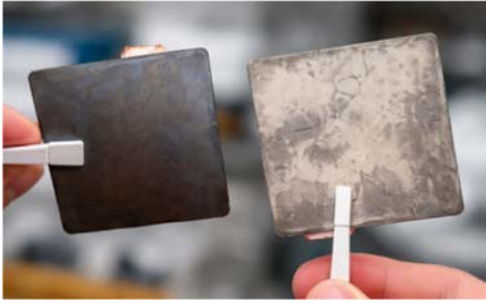
Fig. 1. Lithium plating on a battery electrode; the right electrode shows signs of heavy deposition [2]
